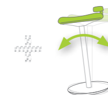
Rocker base. Entire top section can be tilted by up to 7°
